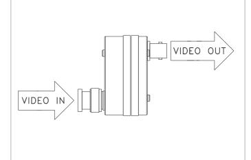
**3.** Once connections have been carried out, green LED ON indicates power supply. Regulate the trimmer in order to adjust the amplification factor until an optimum value of at least 1VPP (CCIR standard) is achieved on screen.
